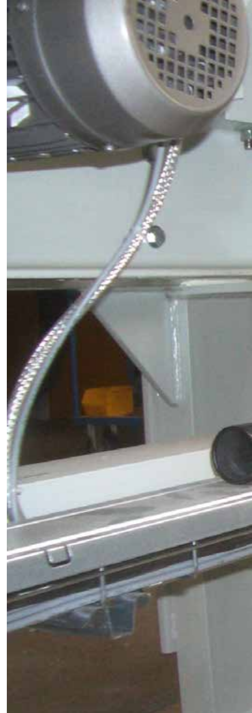
The chain conveyor and the swivel drive of the chain vat are both actuated by two Watt parallel shaft geared motors.
